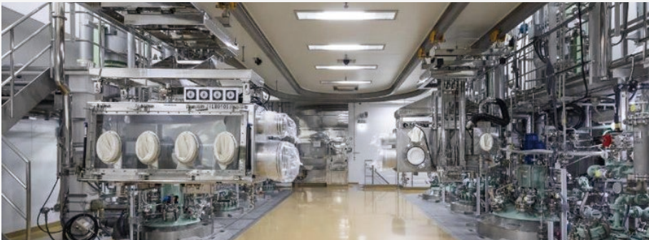
Isolator with containment level of 0.05 µg/m³ or below
