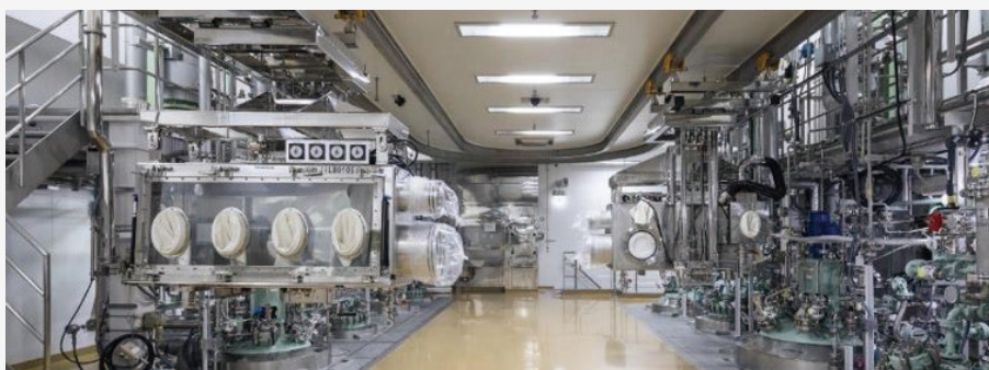
Isolator with containment level of 0.05 \mu\text{g}/\text{m}^3 or below
