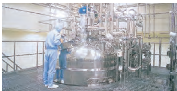
Antibody production cell culture: Cells are transplanted in a 10,000-liter bioreactor for cultivation.
