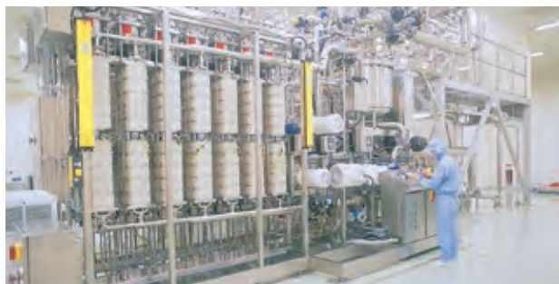
Cell separation: Cells are eliminated from the culture medium.
