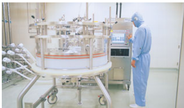
Purification: Impurities are removed with column chromatography to yield high-purity antibodies.
