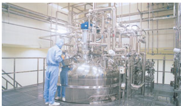
Antibody production cell culture: Cells are transplanted in a 10,000-liter bioreactor for cultivation.
